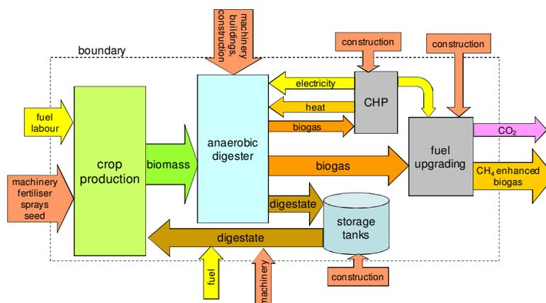
**Figure 4:** Crop based digestion for vehicle fuel - digestate recycled to crop
