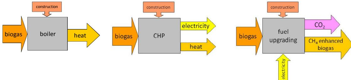
**Figure 3:** Energy and material inputs and outputs post digestion
