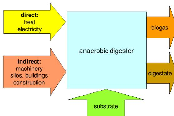
**Figure 2:** Energy inputs and outputs to digestion
